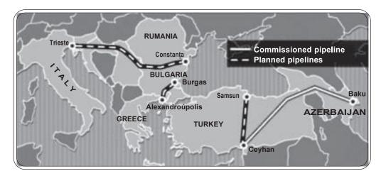
The 1,300-km-long oil pipeline with the annual planned capacity of up to 100 million tons of oil will be completed by 2012; the oil refineries of Italy and Central Europe will receive Kazakh and Azeri oil.
