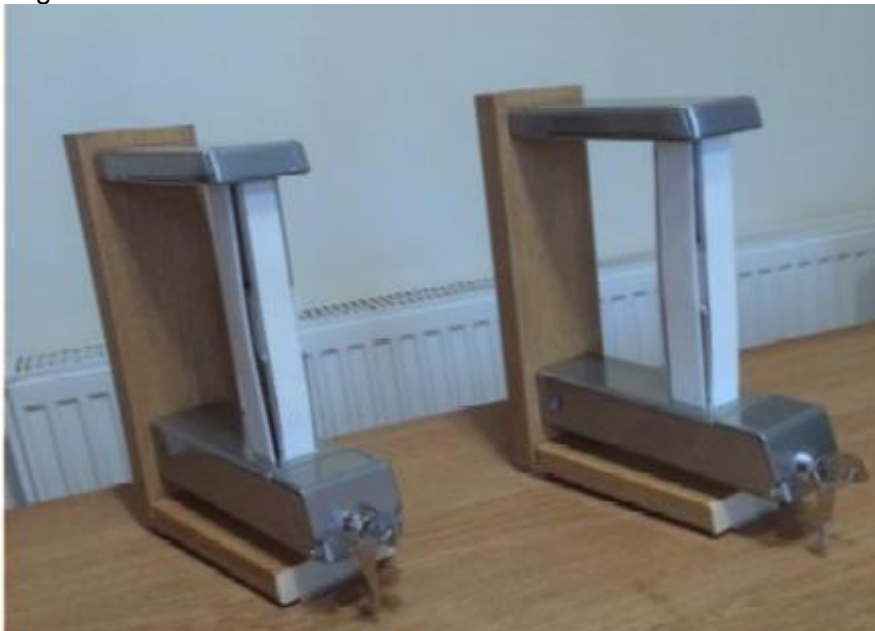
Figure 3.3: Steel framed prototype antimicrobial door handles (Muirhead et al., 2017)
